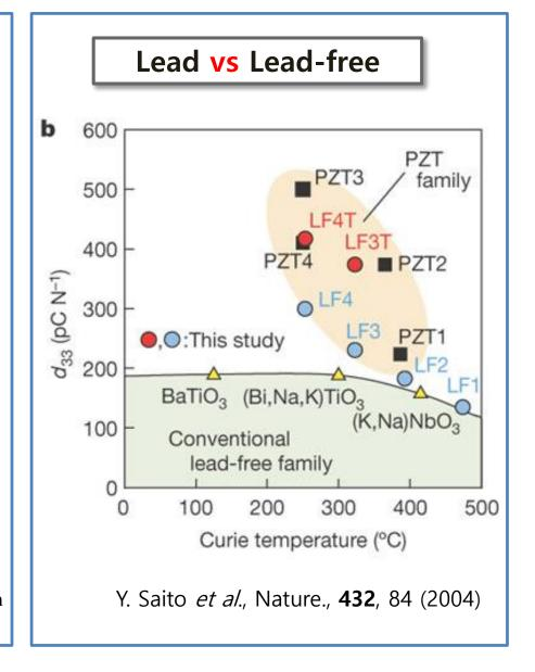
Find a new lead-free piezoelectric materials for replacement of lead-based piezoelectric materials
